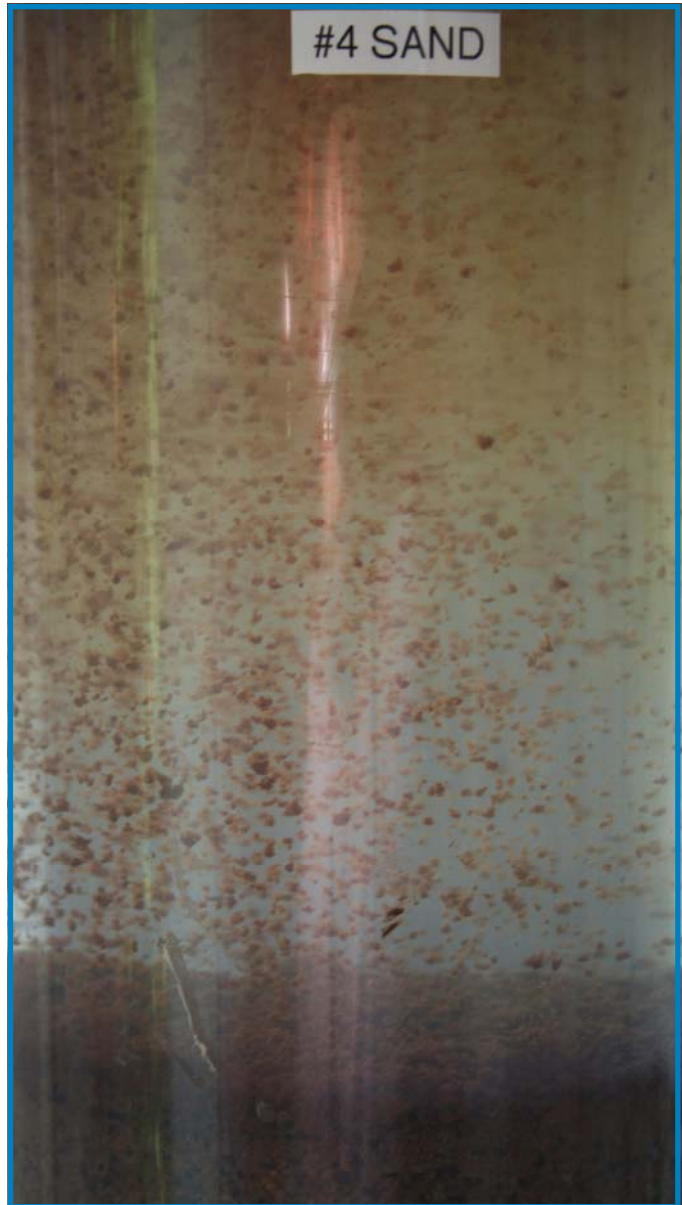
Rising floc from backwashing biological iron filter
